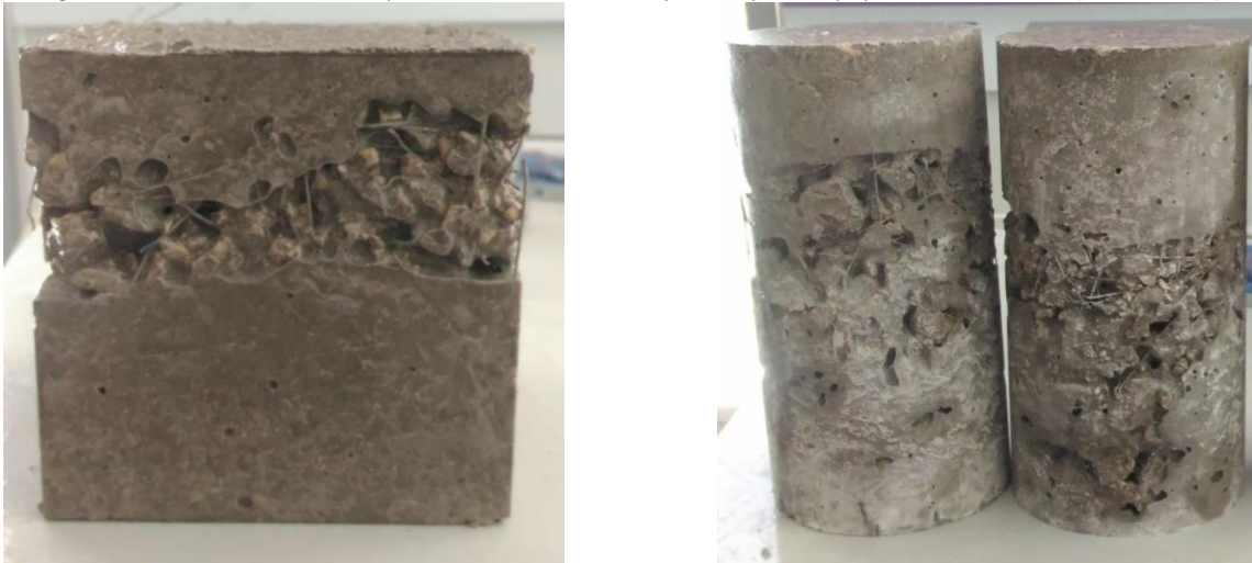
Figure 13. The wall effect of the 10 cm separated cubes and \varnothing 10 \times 20 cm cylindrical specimens prepared with L07 mixtures. (Self-Elaboration).
