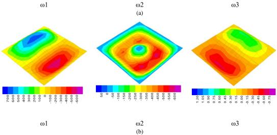
Figure 16. Mode shapes of the two-way slabs (a) two-way slab without column; (b) two-way slab with column.
