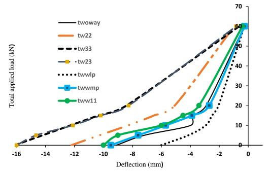
Figure 10. Load-deflection curve for two-way slab without column.
