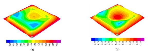
Figure 14. Deflection shape at load level 20 kN (ultimate) (a) slab without column; (b) slab with column.
