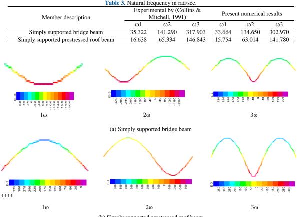
(b) Simply supported prestressed roof beam Figure 4. Mode shapes (a) simply supported bridge beam; (b) simply supported pretressed roof beam.
