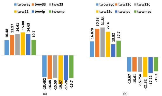
Figure 12. Maximum linear moments at 20 kN uniformly distributed load (a) two-way slab without column; (b) two-way slab with column.
