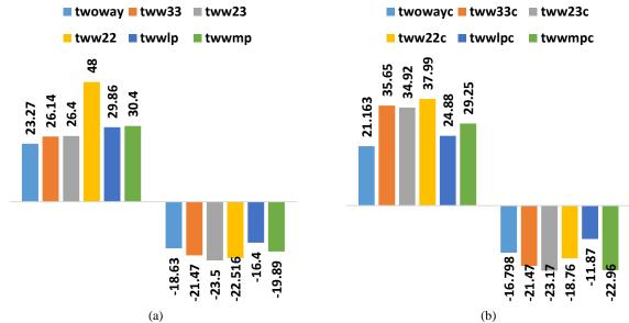
Figure. 13. Maximum nonlinear moments at 20 kN uniformly distributed load (a) two-way slab without column; (b) two-way slab with column.
