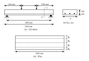
Figure 1. Geometry and arrangement of applied loads of slab 4 and 5 with strands positions.
