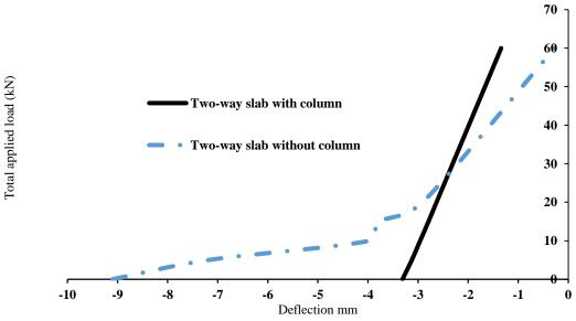
Figure 17. Maximum deflection for the two-way slabs with and without column.
