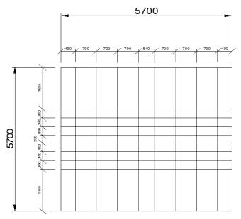
Figure 9. Two-way slab geometry and strand positions.
