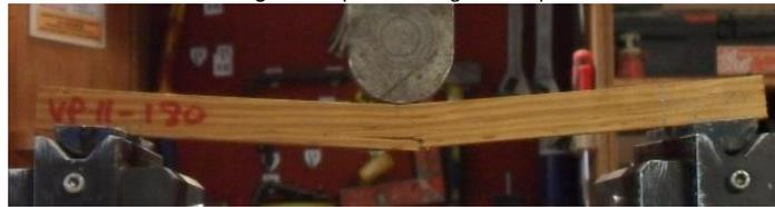
**Table 7.** MoE values (GPa) obtained in 3-point bending tests for all wood species with a  $t_e$  of 2 hours and  $T_{max}$  of 200°C, 240°C, 260°C and 300°C.
