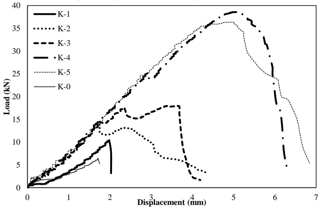
The load-displacement curve of each test sample is given in Figure 6. Figure 6 shows that an improvement in ductility of the samples was observed due to increased fiber ratio. However, after the fiber amount exceeds 4%, reduced strength and reduced energy consumption capacity were observed.
