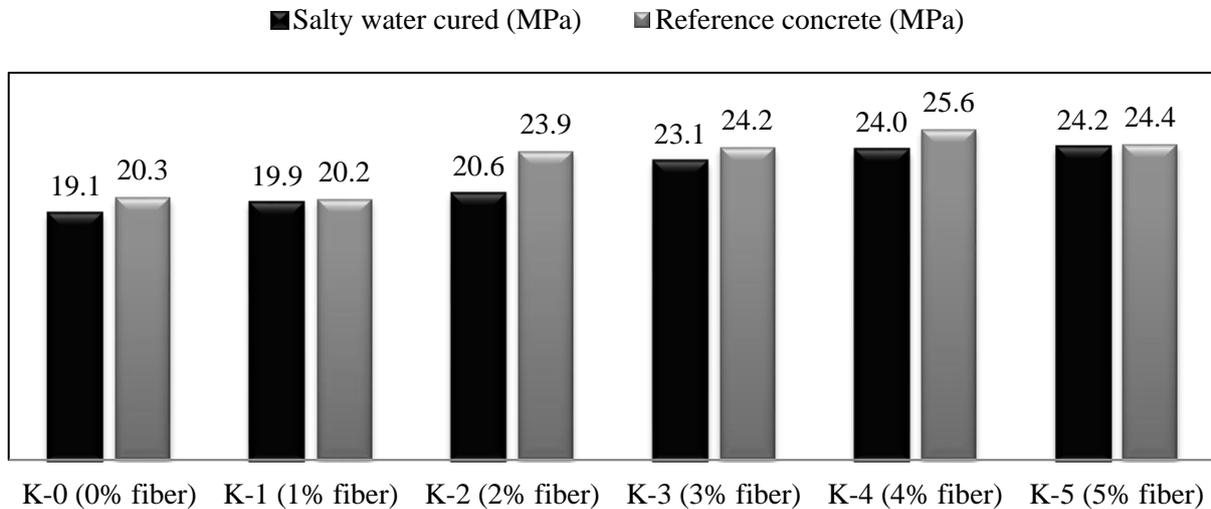
No significant decrease in the strength of concrete is observed as seen in Figure 11. When the specimens compared with that cured in salty water or cured in normal water. Corrosion of steel bead wires are concentrated on the surface of the cubes. Concrete matrix interlocking was observed between corroded steel beads and cement mortar due to increased volume of corroded steel beads. Additionally, salt particles were observed on the surface of the cubes (Figure 12).
