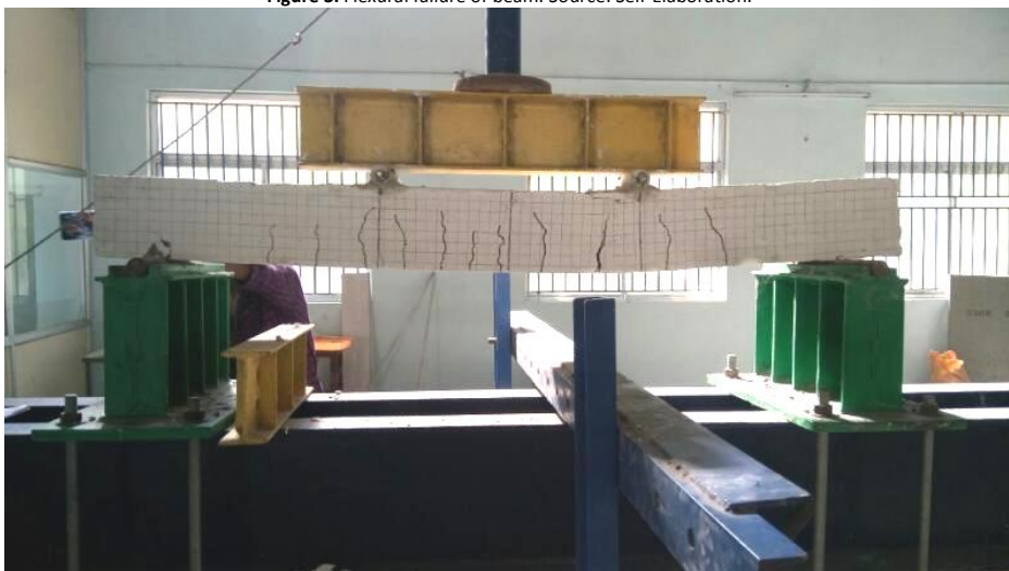
Figure 3. Flexural failure of beam. Source: Self-Elaboration.
