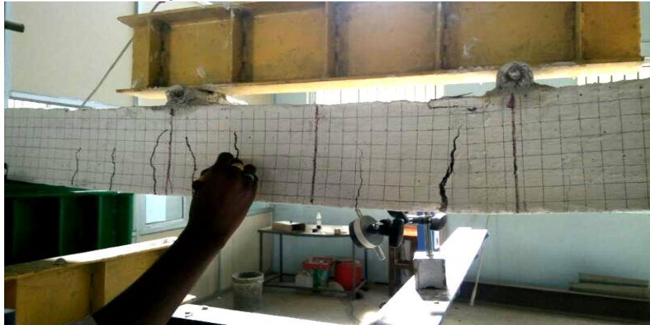
Figure 4. Beam failure at ultimate load. Source: Self-Elaboration.
