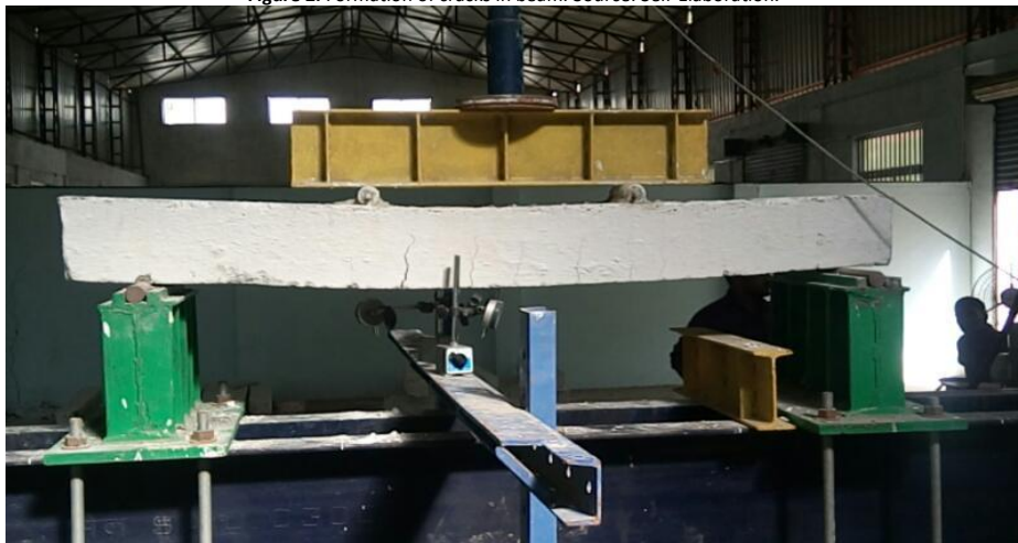
Figure 2. Formation of cracks in beam. Source: Self-Elaboration.
