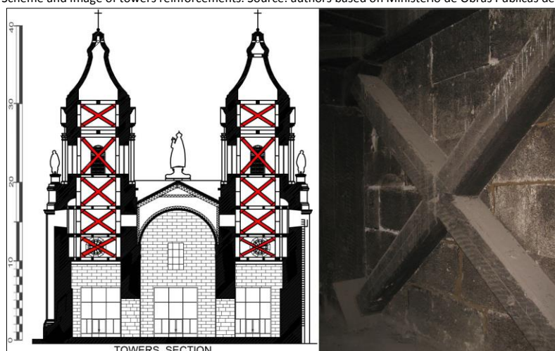
Figure 3. Scheme and image of towers reinforcements. Source: authors based on Ministerio de Obras Públicas de Chile plans.
