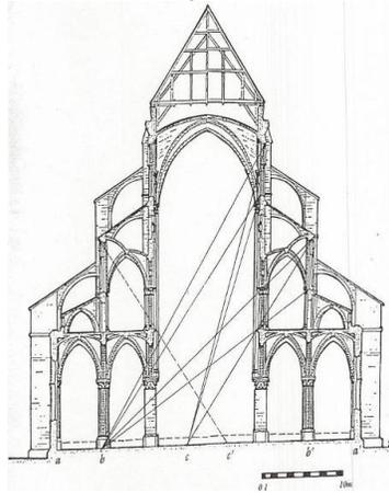
**Figure 4.** Cross section of Toledo's Cathedral, from the entrance of the church. Source: Self-elaboration.
