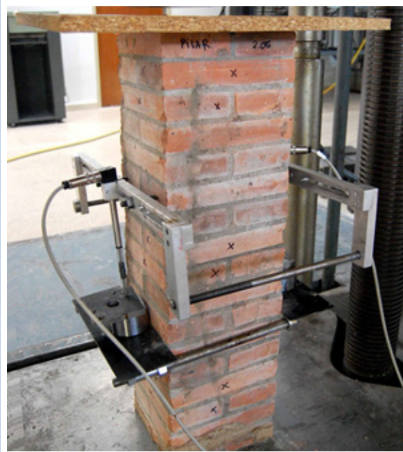
Figure 1. Compressive strength test in columns. Source: self-elaboration.
