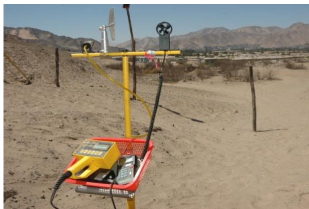
Figure 7. Measurement of direction, wind speed and breathable particulate matter (a) equipment (b) evaluation (PM10 and PM2.5). Source: Self-elaboration, 2010.
