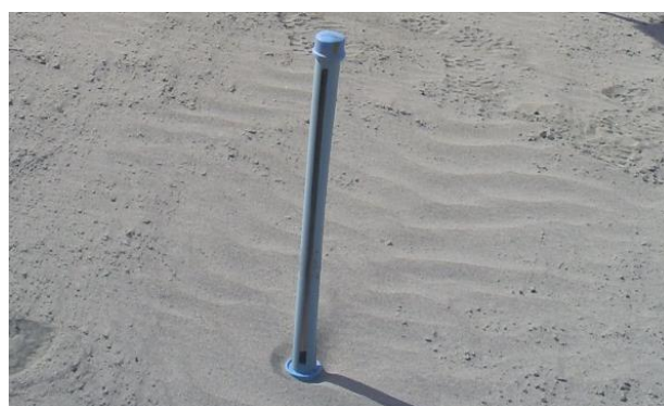
Figure 9. Measurement matter transported by saltation (a) Leatherman trap, (b) evaluation. Source: Self-elaboration, 2010.
