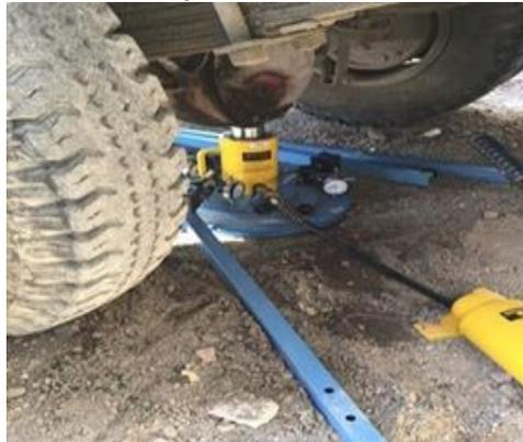
The device was calibrated by national standard organization with coverage factor  $k=2$  correspond to confidence level 95% and the required data were collected after installing equipment, applying load on a steel plate and recording load and settlement rate simultaneously by load and settlement gauges (Barmenkova & Matweeda, 2015).
