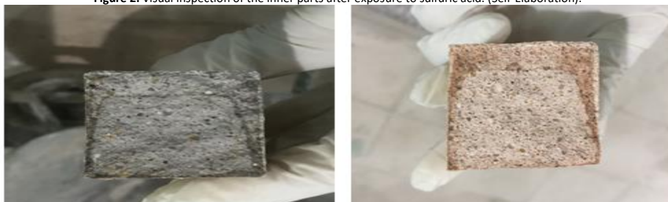
Figure 2. Visual inspection of the inner parts after exposure to sulfuric acid. (Self-Elaboration).
