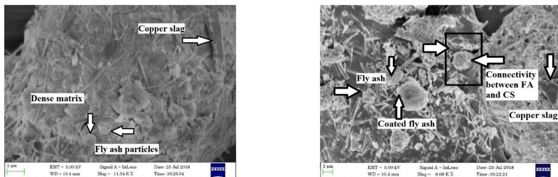
**Figure 16.** FESEM micrographs of 5% Copper slag aggregate incorporated bricks.
