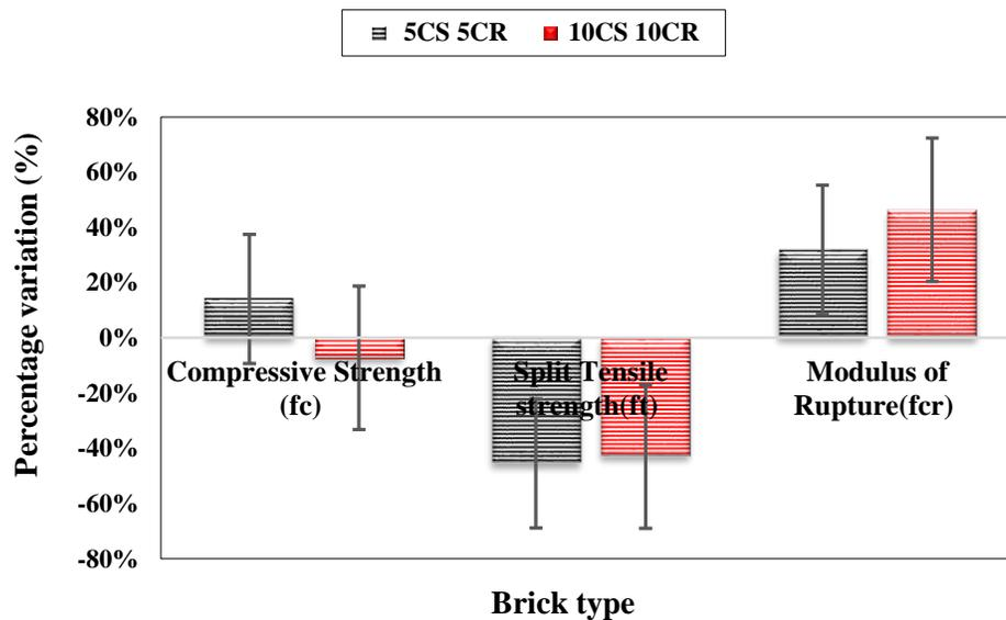
Figure 11. Percentage variation of mechanical properties with the conventional brick mix for the combined substitution of CS and CR at the age of 28 days.
