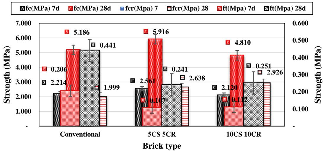
Figure 10. Mechanical properties of combined substitution of CS and CR aggregates.
