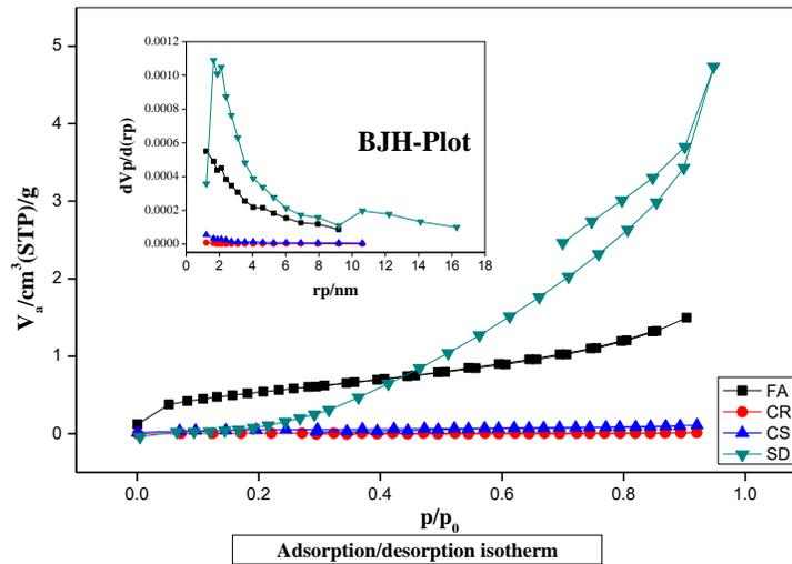
Figure 3. BJH -plot and adsorption/desorption isotherm of ingredients.
