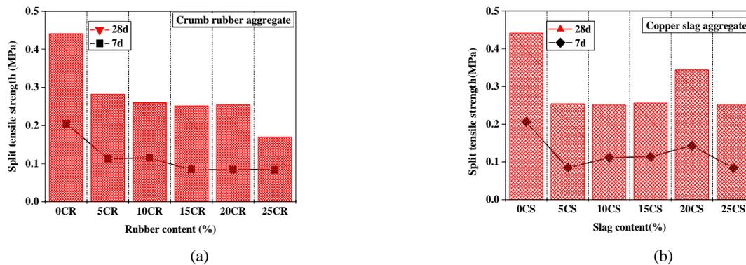
Figure 6. Split tensile strength (a) CR aggregate bricks (b) CS aggregate bricks.
