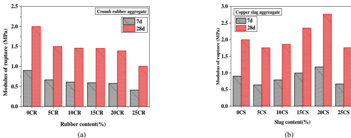
Figure 7. Rupture modulus (a) CR aggregate bricks (b) CS aggregate bricks.
