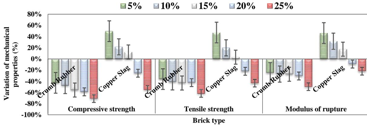
Figure 8. Percentage variation of mechanical properties with the conventional brick mix at the age of 28 days.
