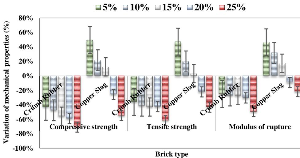
Figure 9. Percentage variation of mechanical properties with the conventional brick mix at the age of 28 days.
