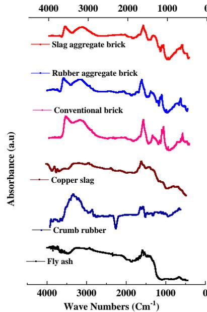
**Figure 14.** FTIR spectra of raw materials and bricks.
