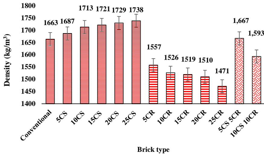
**Figure 4.** Hardened density of bricks incorporating CR and CS aggregates and its combined substitution.
