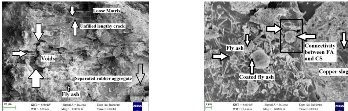
**Figure 15.** FESEM micrographs of 5% Crumb rubber aggregate incorporated bricks.
