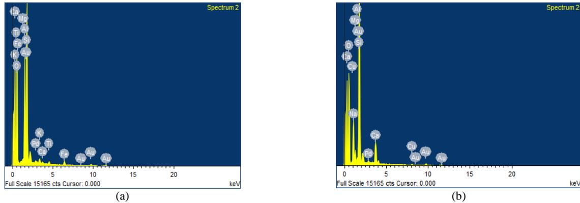
Figure 2. (a) EDS of rubber aggregate; (b) EDS of copper slag aggregate.
