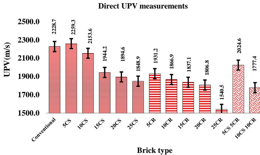
Figure 12. UPV measurements of brick specimens.
