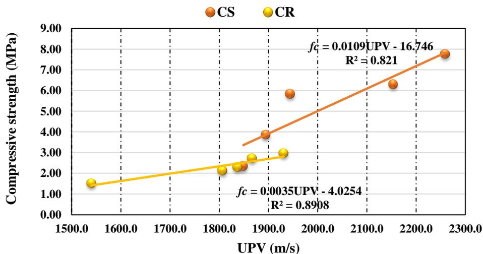
Figure 13. Correlation of UPV and compressive strength of CR and CS aggregate bricks.
