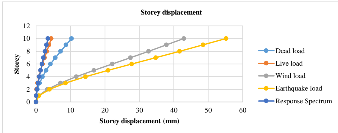
Figure 7. Storey displacement for individual load cases.
