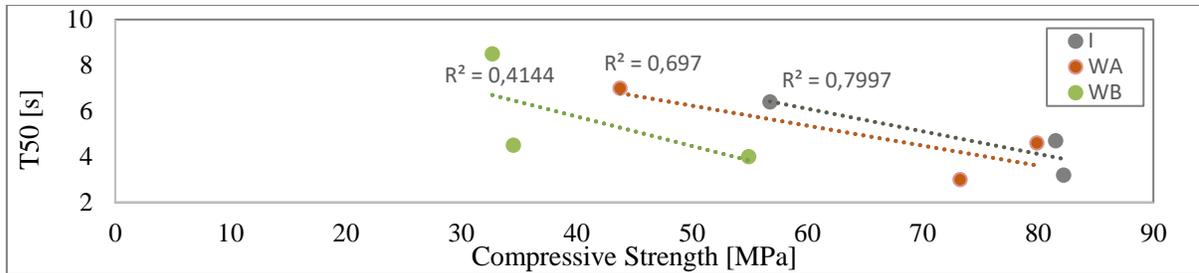
Figure 5. Correlation of compressive strength and T50.
