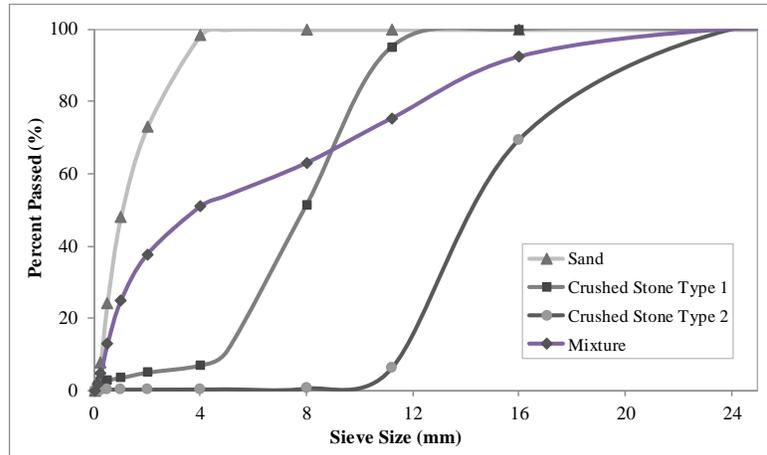
Figure 1. Aggregates grading.
