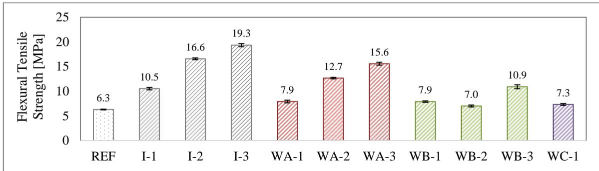
Figure 6. Flexural strength results.
