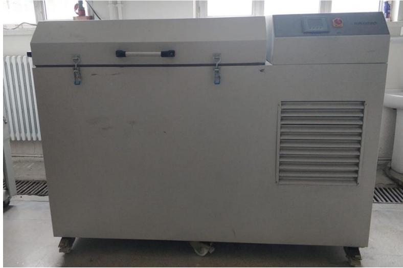
Figure 1. Freeze-thaw test cabin.
