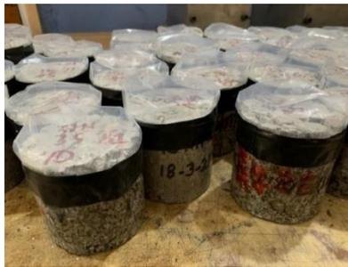
**Figure 9.** Samples for sorptivity test.
