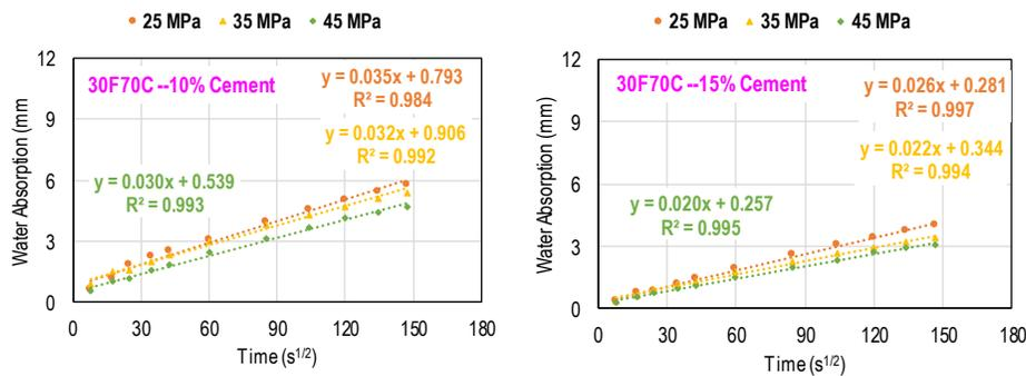
Figure 16. Effect of casting pressure on initial rate of absorption.
