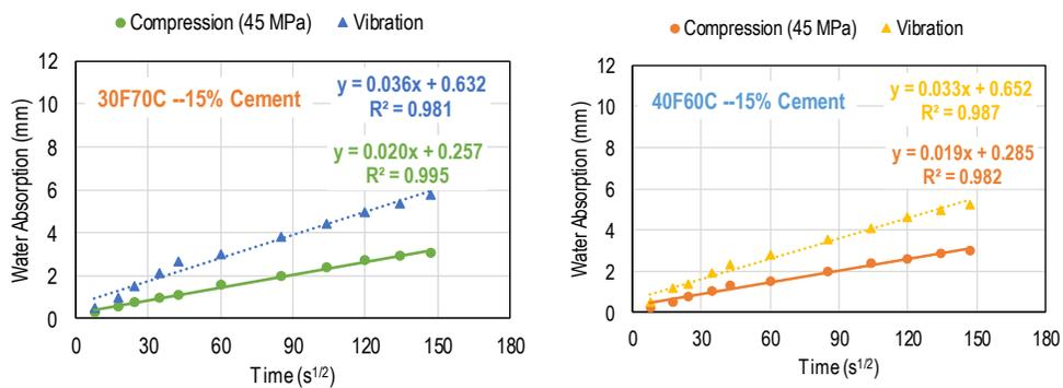
Figure 18. Effect of casting technique on initial rate of absorption.
