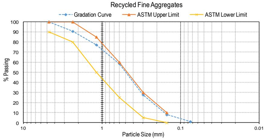
Figure 4. Gradation curve of RFA.
