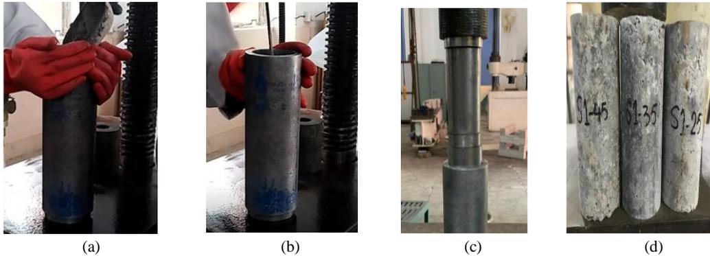
**Figure 8.** (a) Pouring of concrete, (b) manual compaction, (c) compression casting, (d) prepared specimens.
