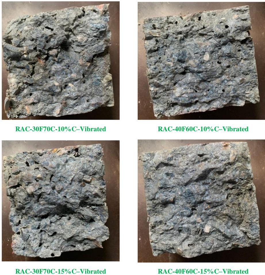
Figure 15. Depth of water absorption after 3 months [vibrated concrete].
