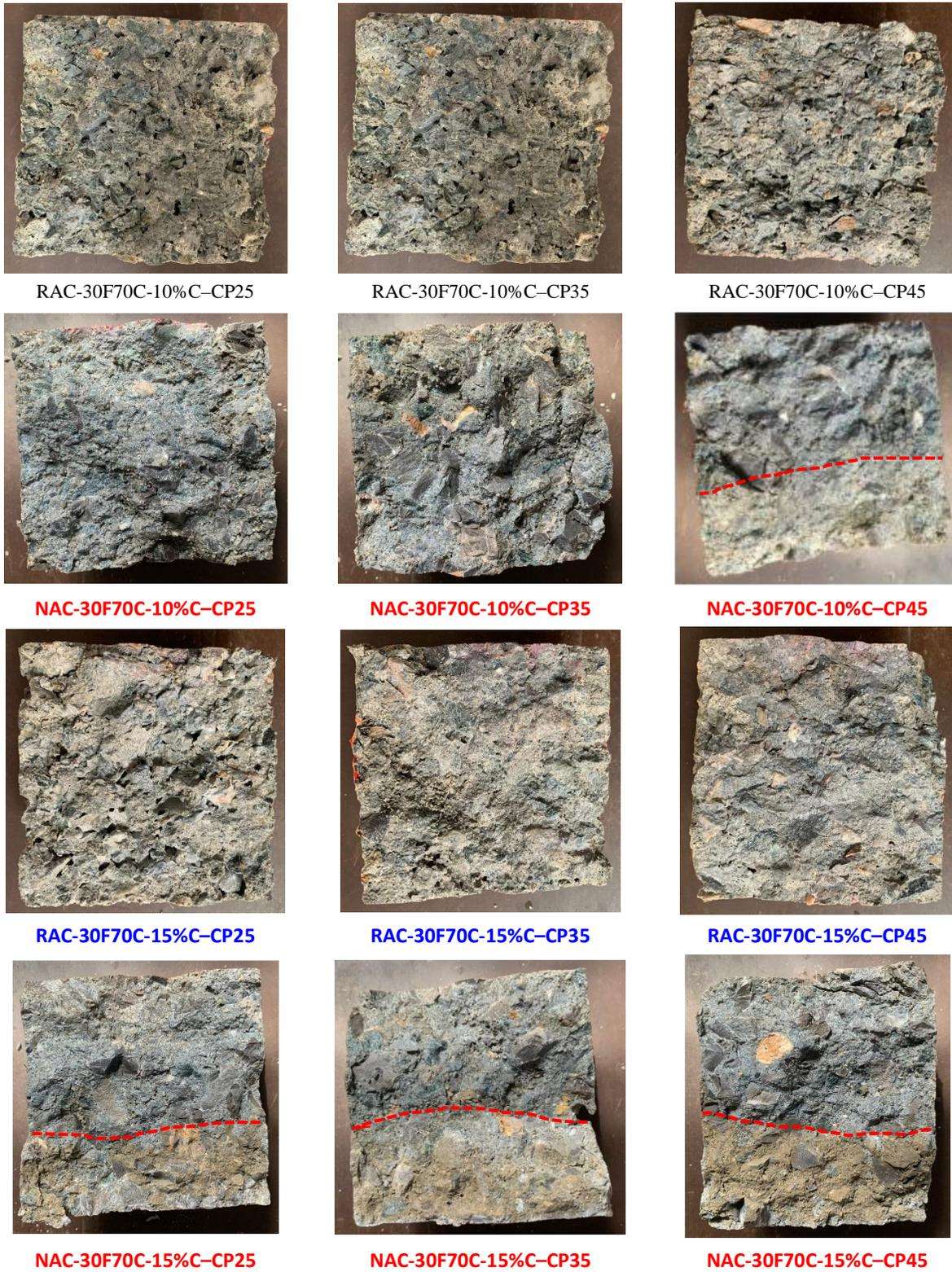
**Figure 13.** Depth of water absorption after 3 months [Mixes 30F70C].
