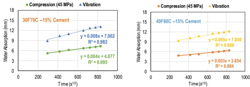
Figure 21: Effect of casting technique on secondary rate of water absorption.
