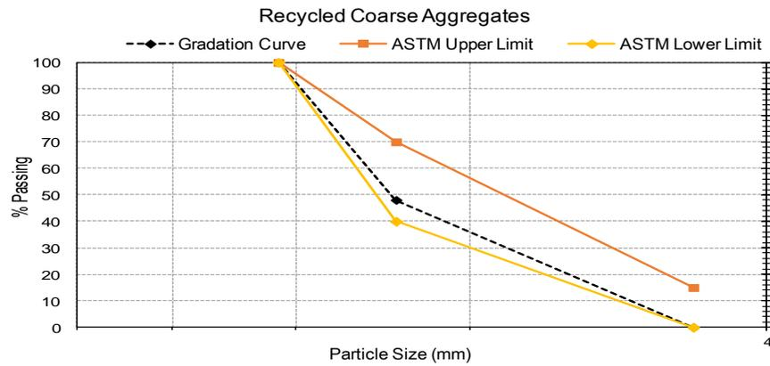
Figure 3. Gradation curve of RCA
