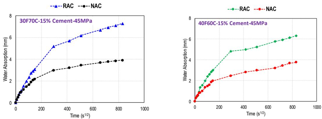
Figure 12. Effect of aggregate type on water absorption.
