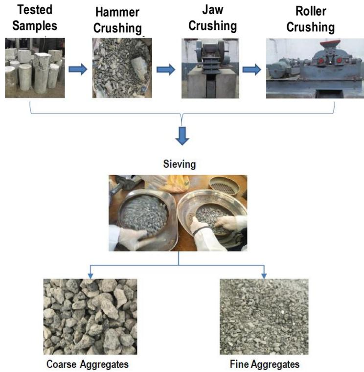
Figure 2. Production process of recycled aggregates.
