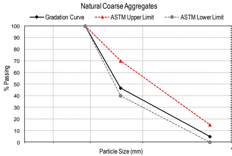
Figure 5. Gradation curve of NCA.
