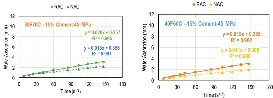
Figure 19. Effect of aggregate type on initial rate of absorption.
