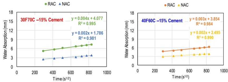
Figure 22. Effect of aggregate type on secondary rate of water absorption.
