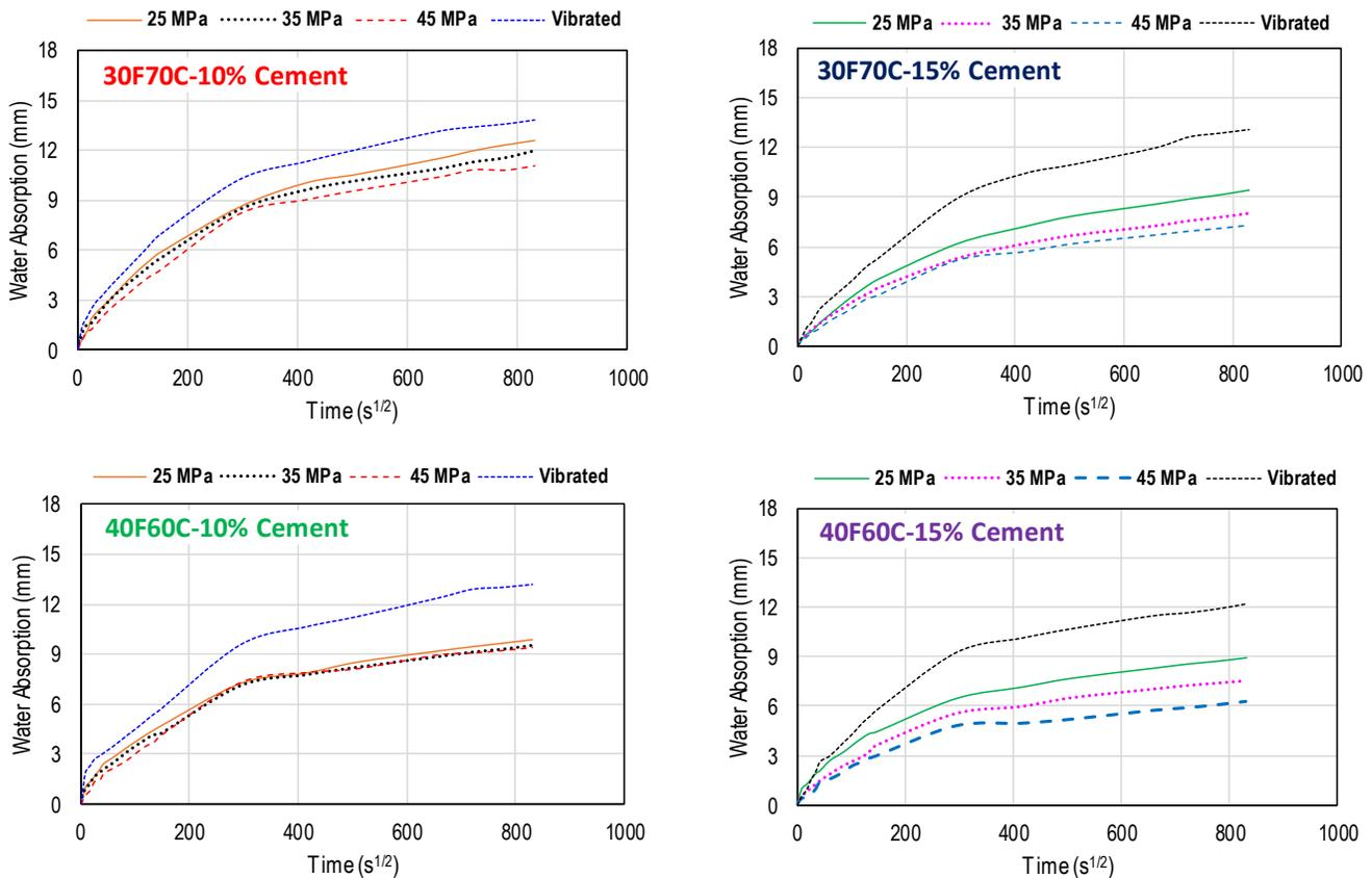
Figure 11. Effect of casting technique on water absorption.
