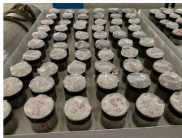
**Figure 10.** Test setup for sorptivity test.
