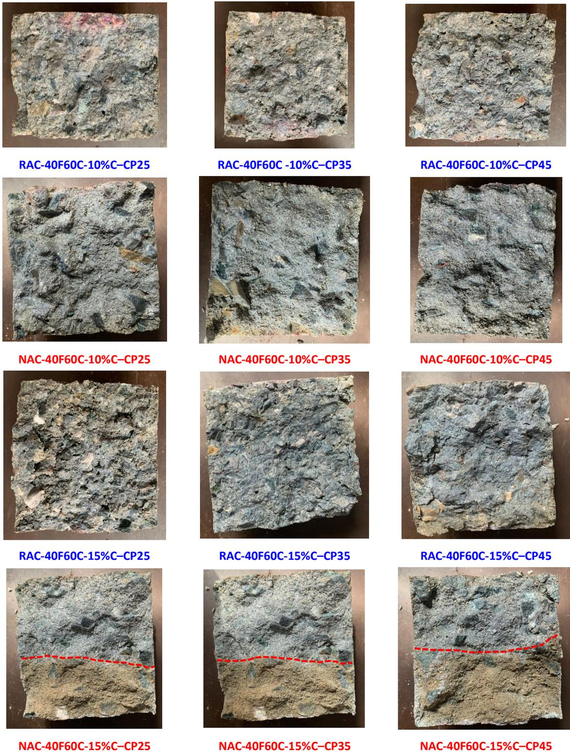
**Figure 14.** Depth of water absorption after 3 months [Mixes 40F60C].
