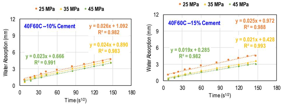
Figure 17. Effect of casting pressure on initial rate of absorption.
