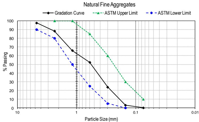
Figure 6. Gradation curve of NFA.
