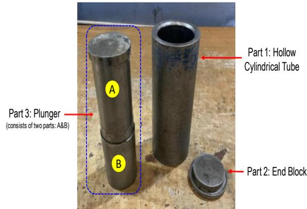
**Figure 7.** Metallic mold prepared for compression casting.
