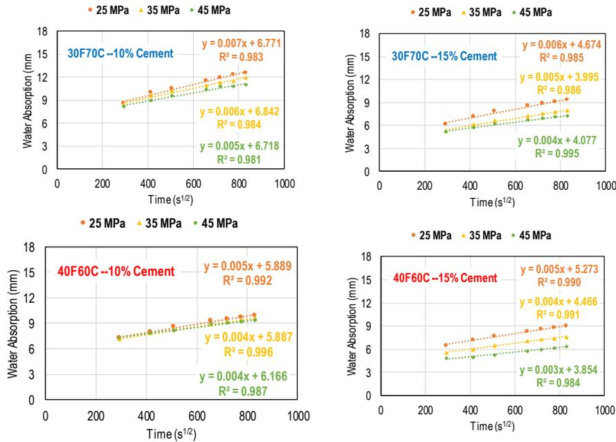
Figure 20: Effect of casting pressure on secondary rate of water absorption.
