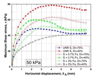
Figure 6. Shear behavior of fiber reinforced sand, shear stress as a function of horizontal displacement, ( $\sigma N=50 \text{ kPa}$ ); Dr=75%: and Dr=40%.
