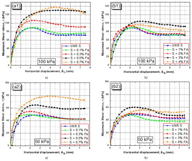
**Figure 4.** Shear behavior of fiber reinforced sand, shear stress as a function of horizontal displacement, ( $\sigma$ N=50 kPa and  $\sigma$ N=100 kPa); Dr=75%: (a) Sisal fiber (Fs), (b) Alfa fiber (FA).
