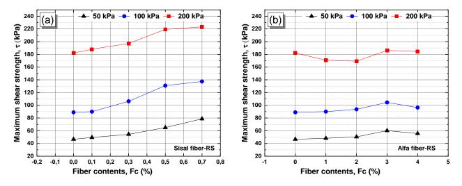
Figure 7. Effect of fiber content on maximum shear strength: (a) Sisal fiber (Fs), (b) Alfa fiber (FA). .1
