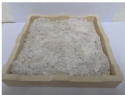
Figure 2. The waste oyster shells after sintering and grinding.
