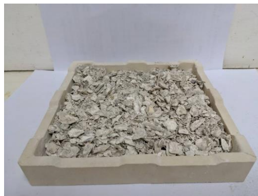
Figure 1. The waste oyster shells before sintering.
