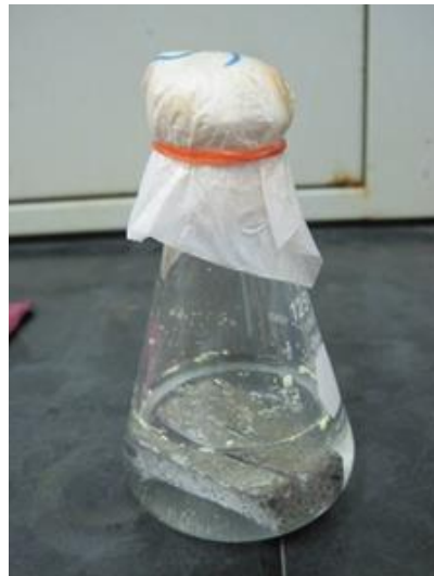
Figure 5. Test piece immersed in the bacterial solution.
