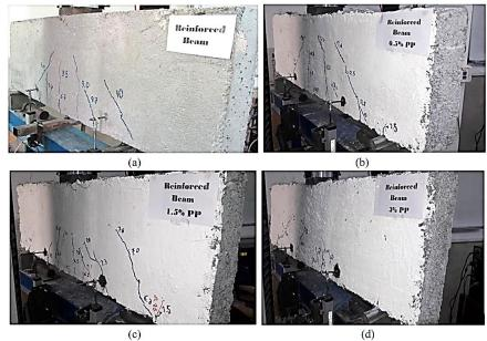
Figure 8. Loading procedure; a) control beam, b) 0.5% PP-R, c) 1.5% PP-R, d) 3.0% PP-R.
