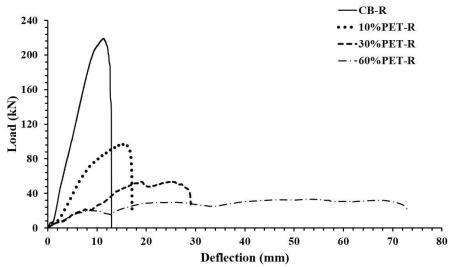
Figure 7. Comparing capacity curve of CB-R, 10% PET-R, 30% PET-R and 60% PET-R beams.
