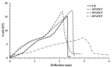
Figure 13. Comparing capacity curve of CB, 10% PET, 30% PET and 60% PET beams.
