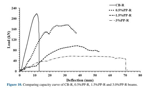
As showed in Figure 10, the shear strength is decreased while the displacement corresponding to the failure point is increased.
