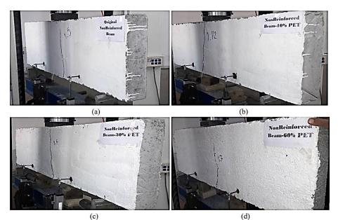
Figure 11. Loading procedure; a) control beam, b) 10 %PET, c) 30%PET, d) 60%PET.
