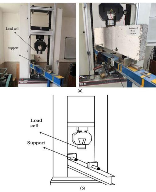
Figure 4. Loading setup; a) real view, b) schematic view.
