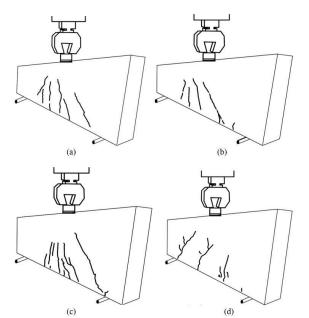
Figure 9. Crack pattern; a) control beam, b) 0.5% PP-R, c) 1.5% PP-R, d) 3.0% PP-R.
