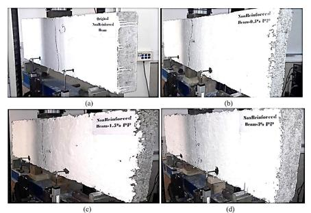
Figure 14. Loading procedure; a) control beam, b) 0.5 % PP, c) 1.5% PP, d) 3.0% PP.
