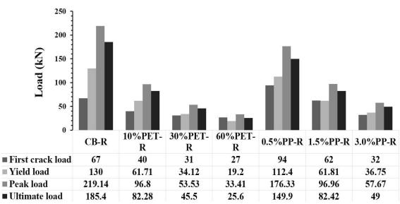
Figure 18. Influence of the PET and PP on the RC beams strength.
