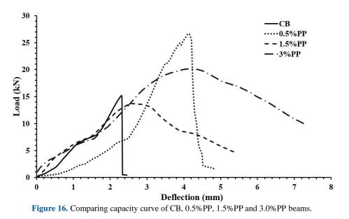
As showed in Figure 16, in the beams with 0.5% and 3% PP, the shear strength is significantly increased and in the beam with 1.5% PP it's decreased. In all the PP dosage the failure displacement significantly is increased.
