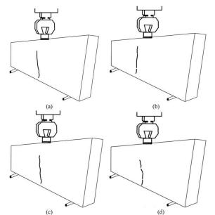
Figure 12. Cracks pattern; a) control beam, b) 10 %PET, c) 30%PET, d) 60%PET.
