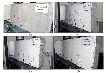
Figure 5. Loading procedure; a) control beam, b) 10% PET-R, c) 30% PET-R, d) 60% PET-R.
