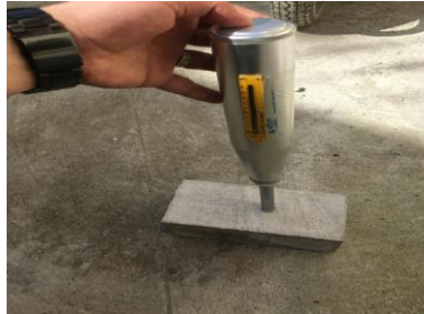
Figure 5. Surface hardness measurement on pavings with the Schmidt test hammer.
