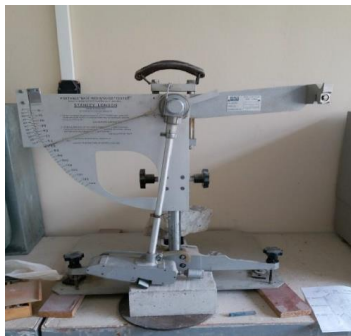
Figure 4. Pendulum friction test equipment.
