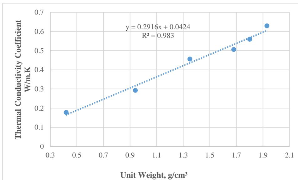
Figure 13. The relationship between thermal insulation and unit weight.
