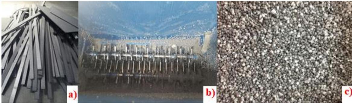
**Figure 1.** Pictures of waste EPS a) the waste EPS pieces b) graining process c) waste EPS aggregates.
