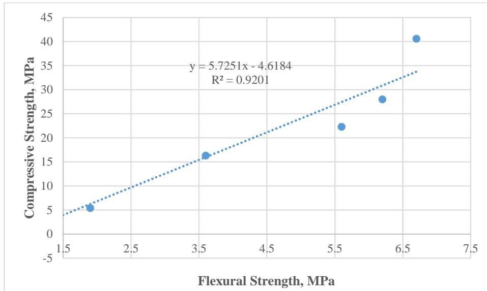
**Figure 10.** The relationship between compressive and flexural strength.
