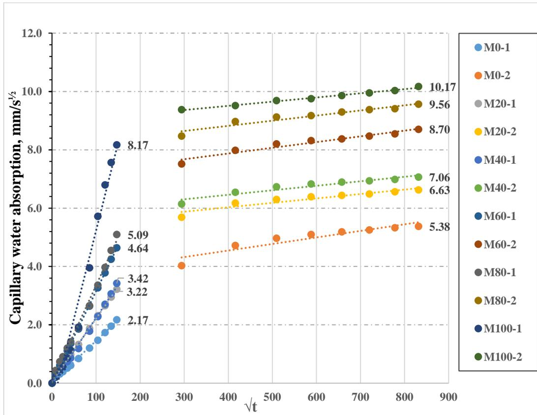
Figure 7. Capillary water absorption test results.
