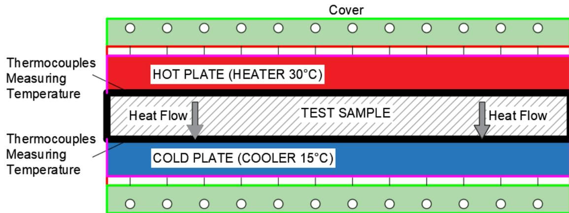
Figure 4. Hot plate device graphic configuration.
