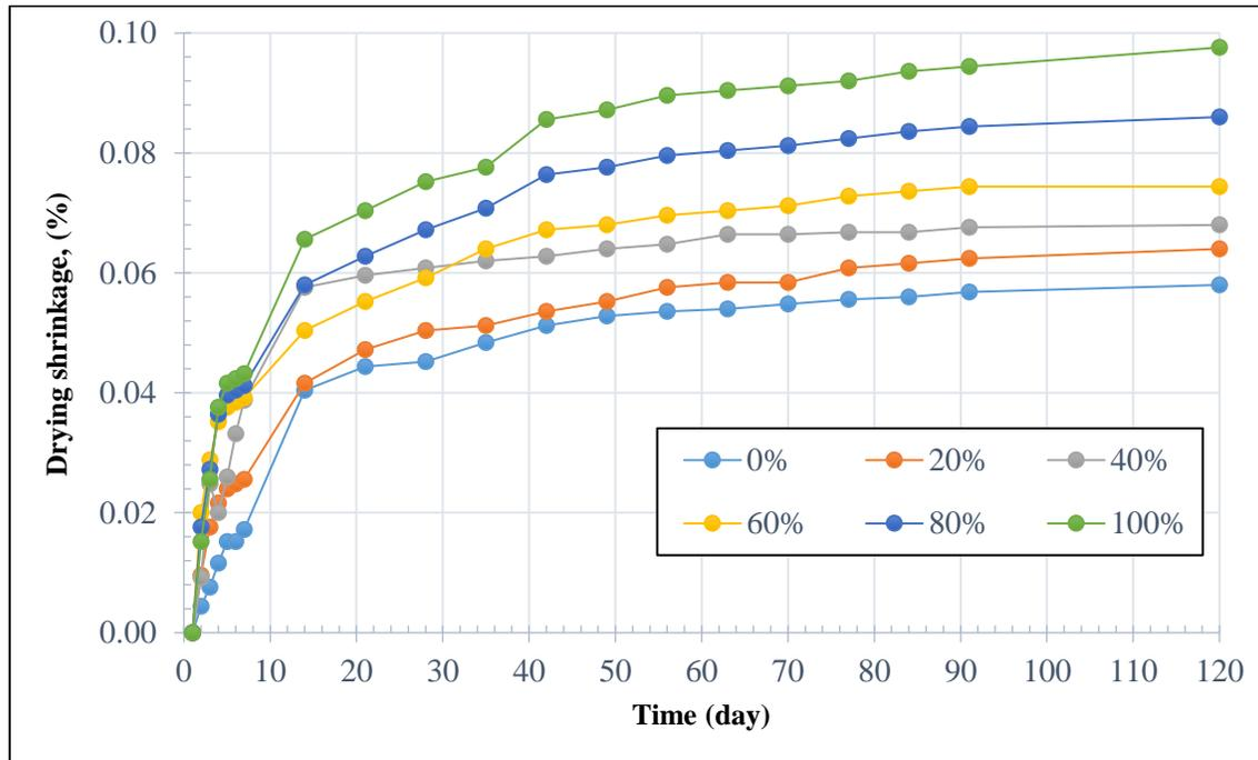
Figure 11. Drying shrinkage results.
