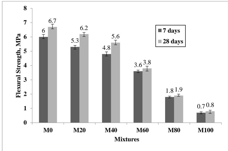
Figure 8. Flexural strength results.
