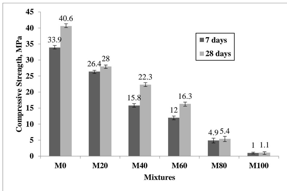
Figure 9. Compressive strength results.
