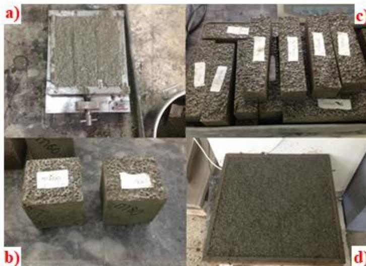
**Figure 2.** View of the prepared specimens a) the mortar mixture placed in the prism mold b) the 100×100×100 mm cube c) the 40×40×160 mm prism specimens d) the 500×500×50 mm plate.
