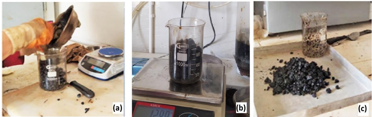
Figure 3. Schellenberger bitumen drain down test.
