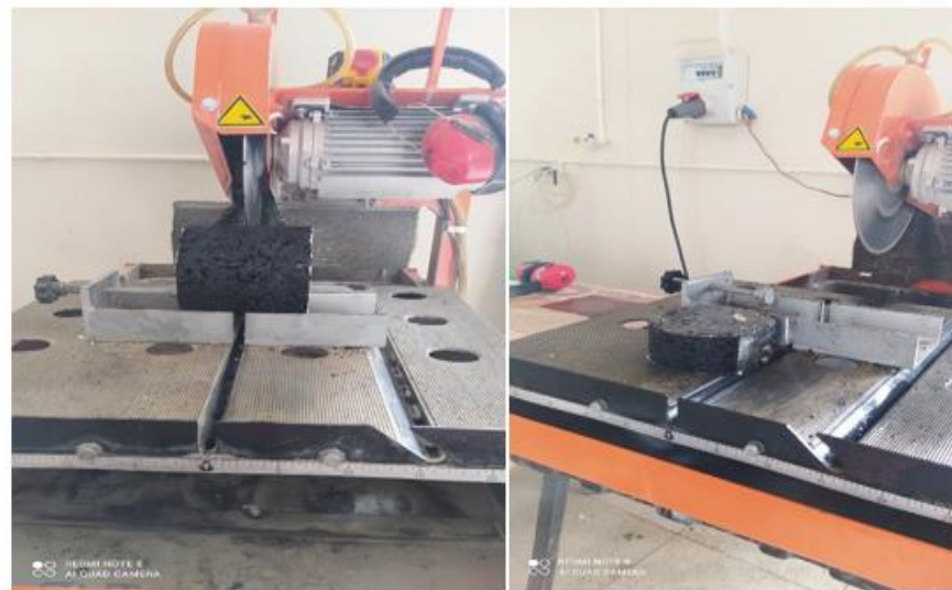
Figure 5. Mixtures cut with an asphalt-cutting machine.
