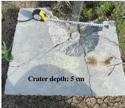
Figure 22. The crater depth of PCC exploded with 150 g TNG.
