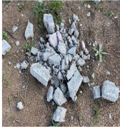
Figure 30. 5% CFGC slab after the explosion with 250 g TNG.
