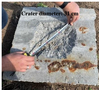
Figure 20. The crater diameter of 5% CFGC exploded with 150 g TNG.
