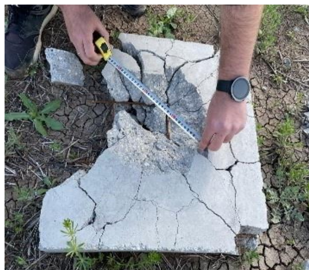
Figure 39. 10% CFGC slab after explosion with 200 g TNG.
