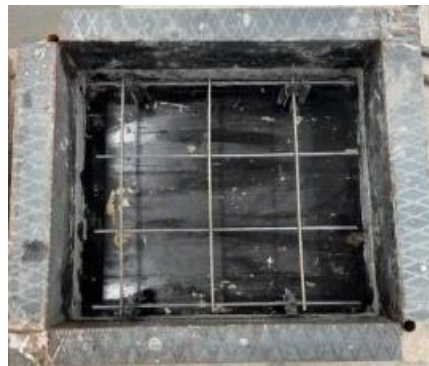
Figure 2. Casting mold (internal dimensions: 50 x 50 x 10 cm).
