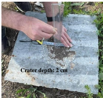
Figure 16. The crater depth of PCC exploded with 100 g TNG.
