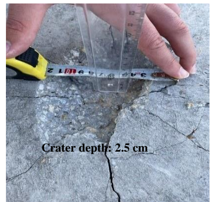
Figure 18. The crater depth of 10% CFGC exploded with 100 g TNG.
