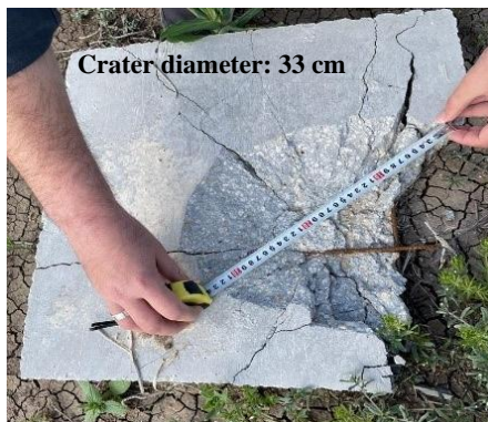
Figure 19. The crater diameter of PCC exploded with 150 g TNG.
