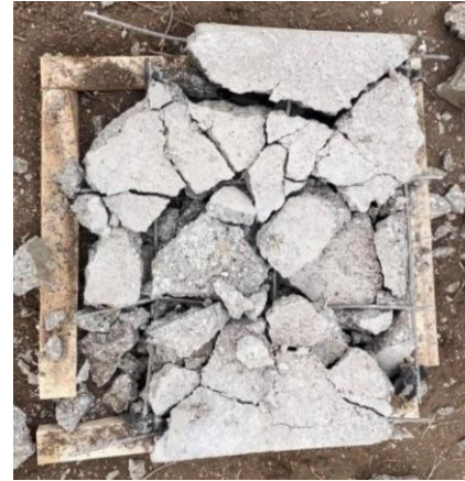
Figure 31. 10% CFGC slab after explosion with 250 g TNG.
