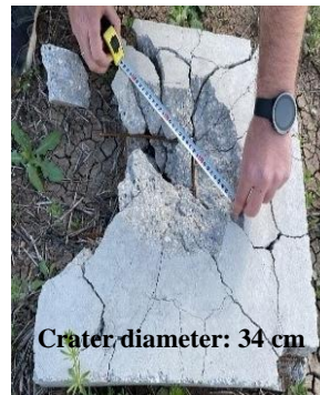
Figure 27. 10% CFGC crater diameter after detonation with 200 g TNG.
