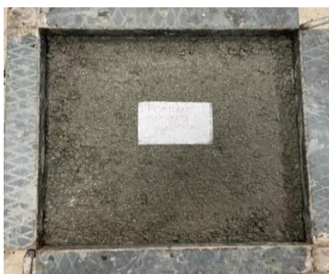
Figure 3. Blast test specimen with PCC content.
