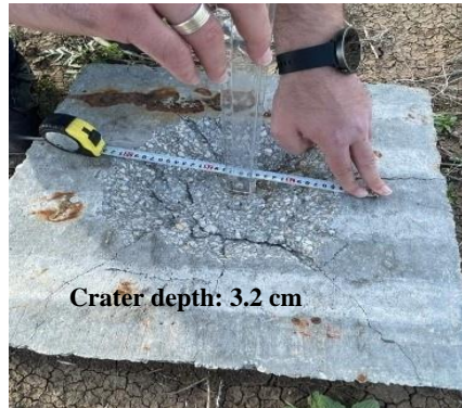
Figure 23. The crater depth of 5% CFGC exploded with 150 g TNG.
