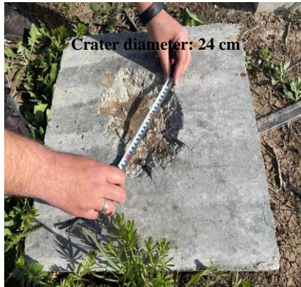
Figure 13. The crater diameter of PCC exploded with 100 g TNG.
