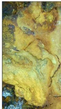
The micrographs show the presence of ferrous oxide and ferric oxide as proof of advance chemical and mechanical mechanisms of damage due to a constant moisture condition.
