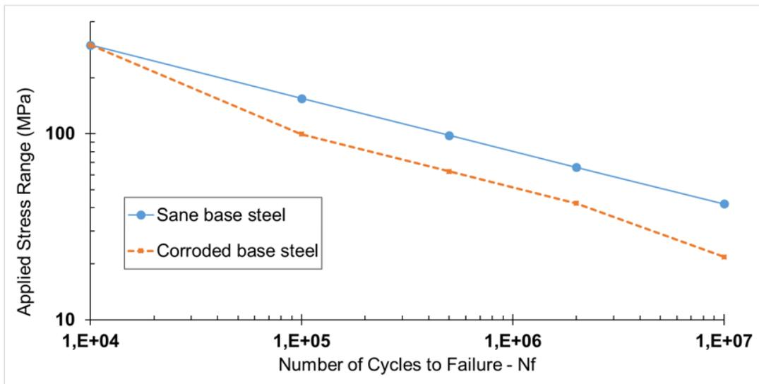
**Figure 8.** Fatigue S-N curve for structural detail No 7 (Ang & Munse, 1975), which is affected by corrosion according to the visual inspection and the micrographs available. Corrosion is assumed to happen in a non-salty environment
