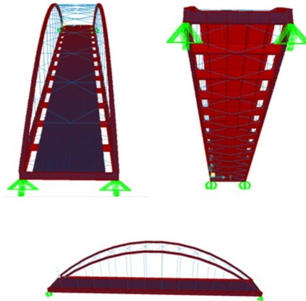
**Figure 9.** Finite element model for the structural elements of the Unete steel arch bridge. Hangers, nodal and relative stiffener models used linear frame elements whereas the rest of the structural elements used shell elements
