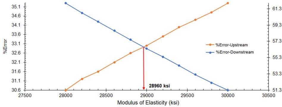
**Figure 14.** Systematic variation for the Unete steel bridge modulus of elasticity. Reported errors between the measured point of control vertical displacement and the simulated vertical displacement
