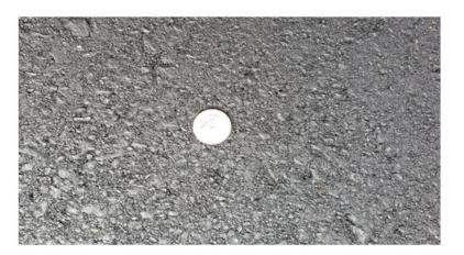
Figure 7. Surface damage for CDD=0 °C-days
