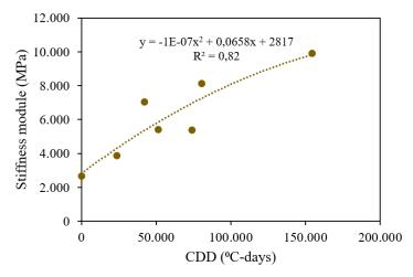
Figure 5. Variation of stiffness modules versus the CDD
