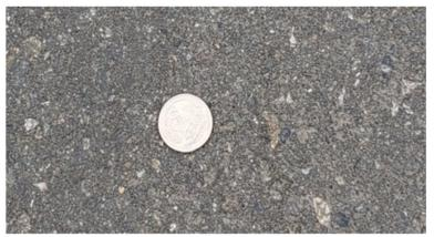
Figure 9. Surface damage for CDD=42.079 °C-days
