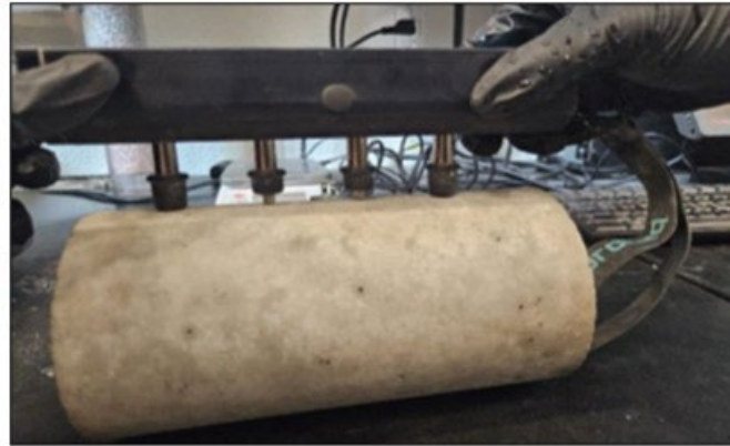
Figure 4. Surface Electrical Resistivity Set-up.
